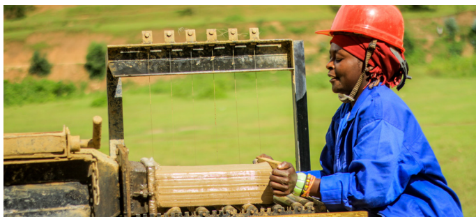
Regulated moisture in the clay column during extrusion for proper handling
