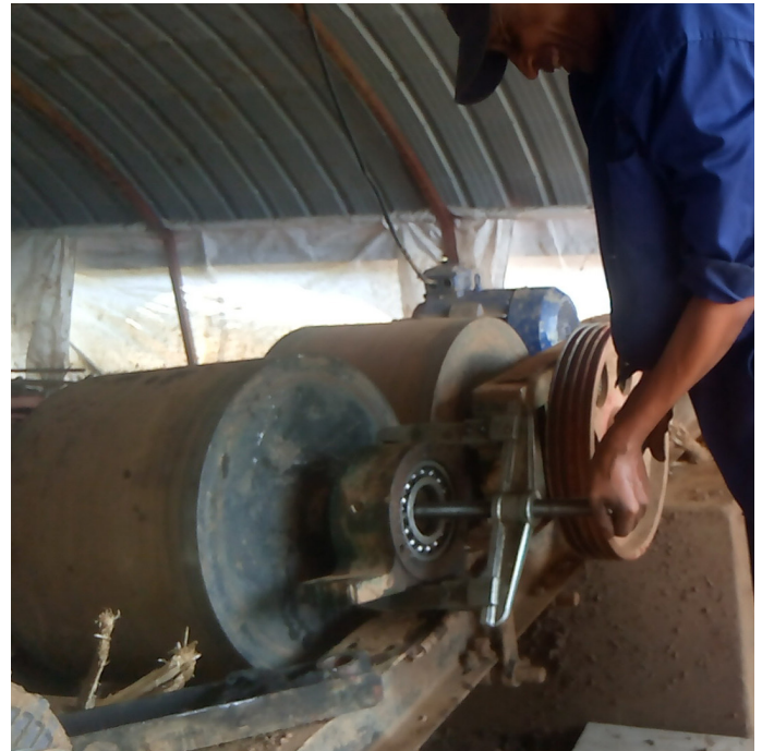
Screw shaft with new full pitch distance
