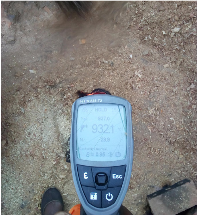
Firing temperature monitoring using a temperature gun
