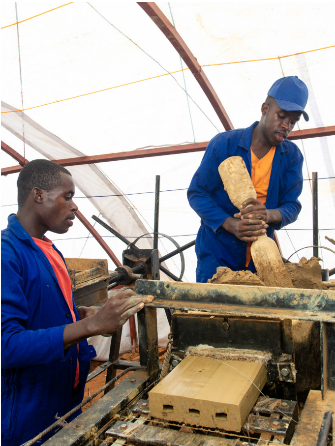
Demonstration of clay box feeding of manual extruder
